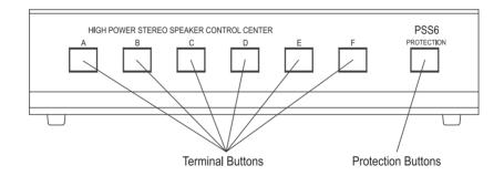
The control center lets you use one to four (PSS4) or six (PSS6) sets of speakers at a time, and is designed to operate with a stereo receiver/amplifier that has a maximum of 100 watts per channel, and with speaker systems that have a minimum impedance of 8 ohms (see "Impedance Chart" on page 5)
