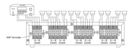
Press open the AMP terminals on the control center, then insert your receiver/amplifier's positive (+) wires into the positive (red) terminals, and negative (-) wires in the nagative terminals. Then press the tabs to close them.
