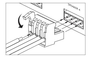
Figure 3 Connecting the Wires
